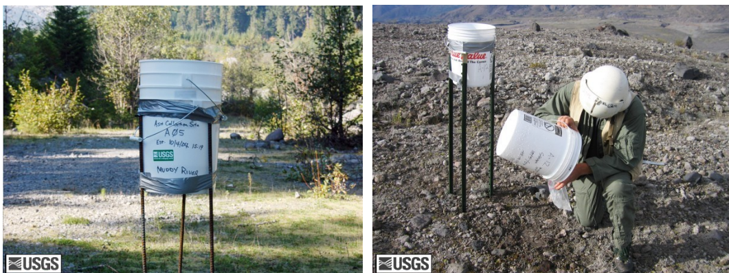
Fig. 1 & 2. Ash collection buckets used by the USGS.
